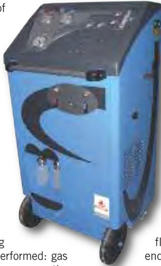
of the process and the onboard printer then produces a comprehensive system diagnosis including gas recovery, oil injection and gas filled in the vehicle.
