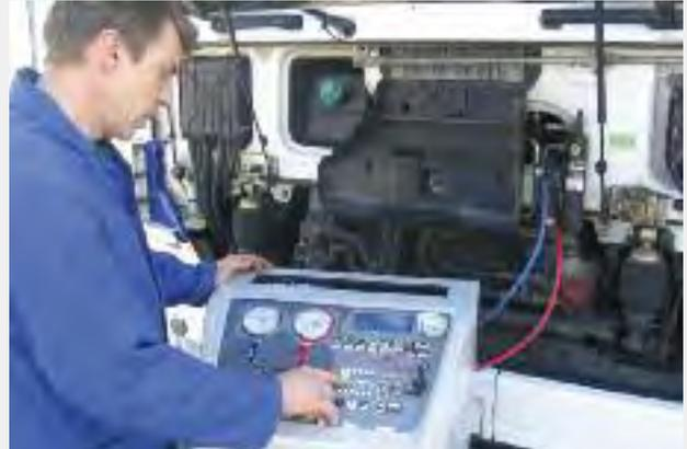
According to the thermal management experts at Behr Hella Service, regular inspection and servicing of commercial vehicle air-conditioning units, (at least every six months), not only saves on costs and time-consuming repairs, but also reduces idle times and downtimes. Regular servicing also reduces the fuel consumption caused by the air-conditioning system.
